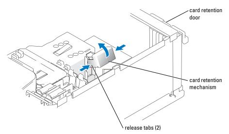
**2** Gently push the release tab on the card retention door from the inside to pivot the door open. Because the door is captive, it will remain in the open position (see "Installing a PCI Card" on page 73 for an illustration of the card retention door).
