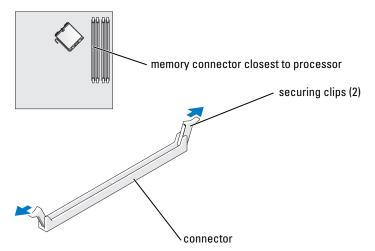
4 Align the notch on the bottom of the module with the crossbar in the connector.
